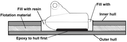
Epoxy the transducer to a solid portion of the hull.
